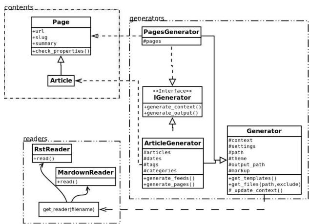
The interface does not really exist, and I have added it only to clarify the whole picture. I do use duck typing and not interfaces.
